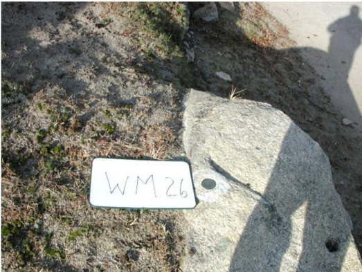
BM WM26 Disk on top of Granite Ledge Outcrop.
