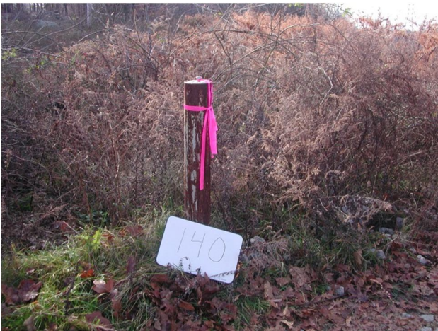
BM 140 Brass Rivet on top of Concrete post inside of metal post.
