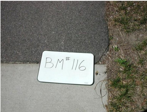
BM 116 Rivet on top of Concrete sidewalk.
