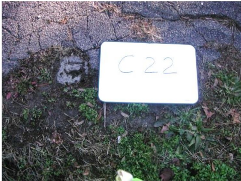
BM C22 Square Cut on top of Granite Bound.
