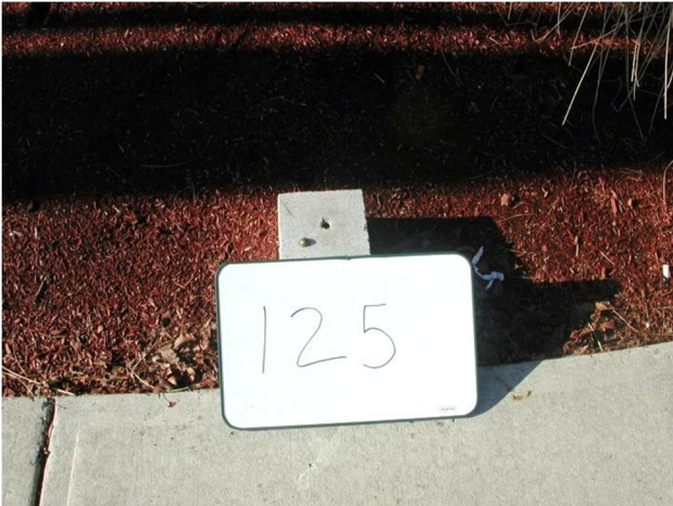
BM 125 Brass Rivet on top of Granite Bound.
