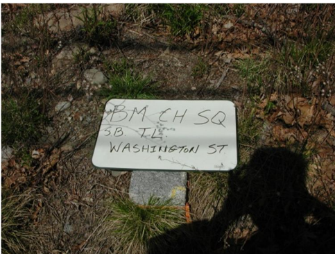
BM CHSQRSB ~ Chiseled Square Stone Bound @ Town Line on Washington St.
