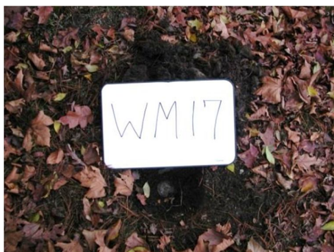
BM WM17 Disk on top of Concrete Bound.
