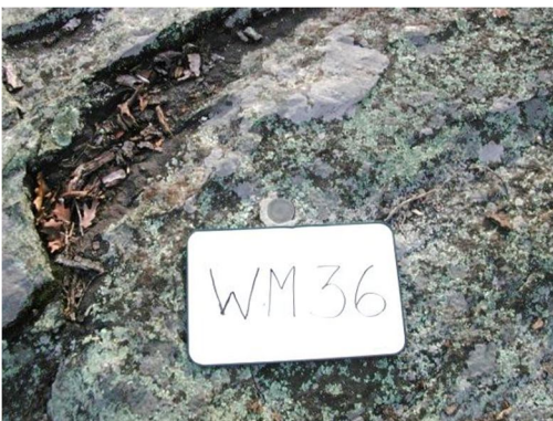
BM WM36 Disk on top of Granite Ledge Outcrop.
