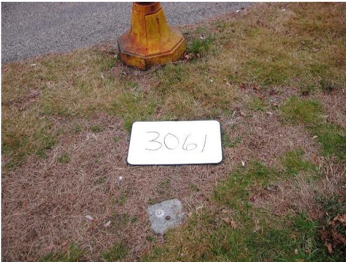
BM 3061 Rivet on top of Stone Bound Monument.
