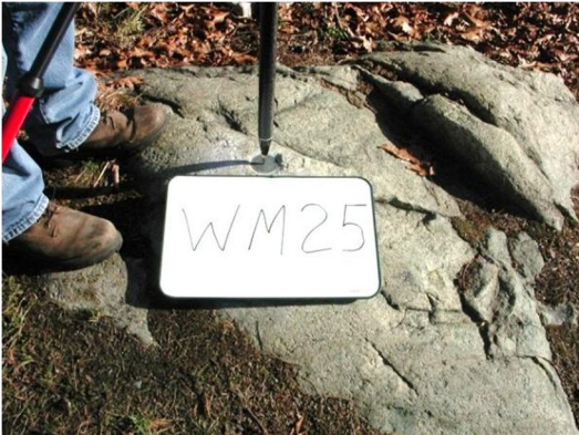
BM WM25 Disk on top of Granite Ledge Outcrop.
