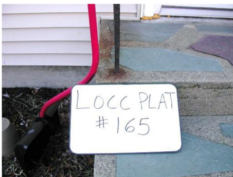
BM LOCC PLAT 165 ~ Left Outer Corner Conc. Platform @ HSE.#165 Green St..
