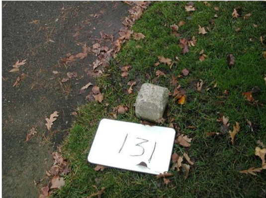
BM 131 Excussion Pin in Lead Plug in Concrete Bound @ Ledgebrook Rd. & Hickory Ln.
