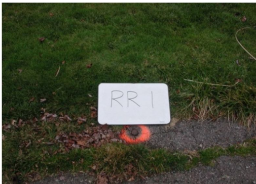
BM RR1 Rail Road Spike in Bituminous Concrete Berm Tilden Circle.
