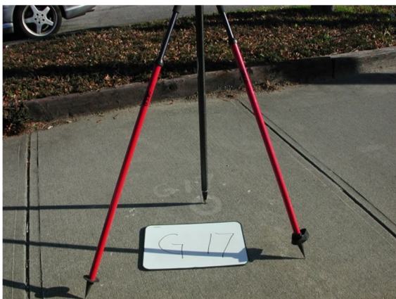
BM G17 Drill Hole in Concrete sidewalk.
