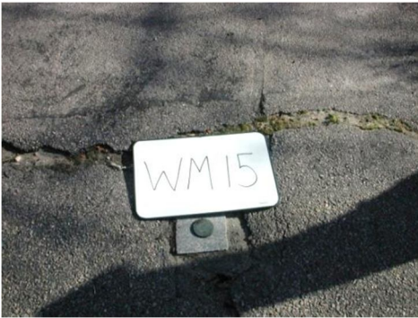
BM WM15 Disk on top of Granite Bound.
