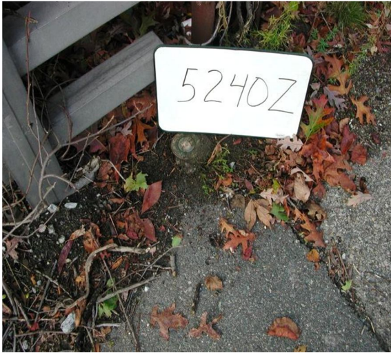
BM 5240Z Disk on top of Concrete.
