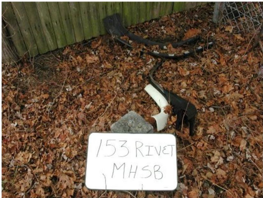
BM 153 Rivet on top of Granite Mass Highway Stone Bound.
