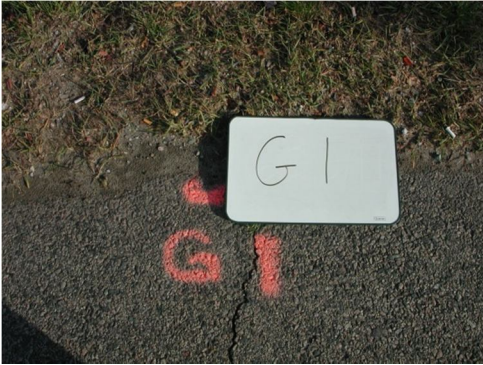
BM G1 Spike in bitumimous Concrete Pavement.
