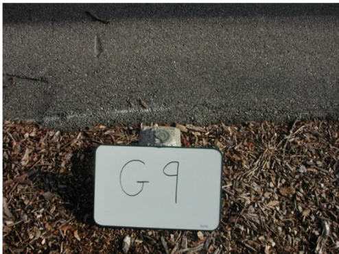
BM G9 Disk on top of Concrete Bound.
