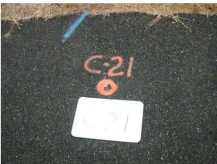
BM C21 Rail Road Spike in Bituminous Concrete Pavement.
