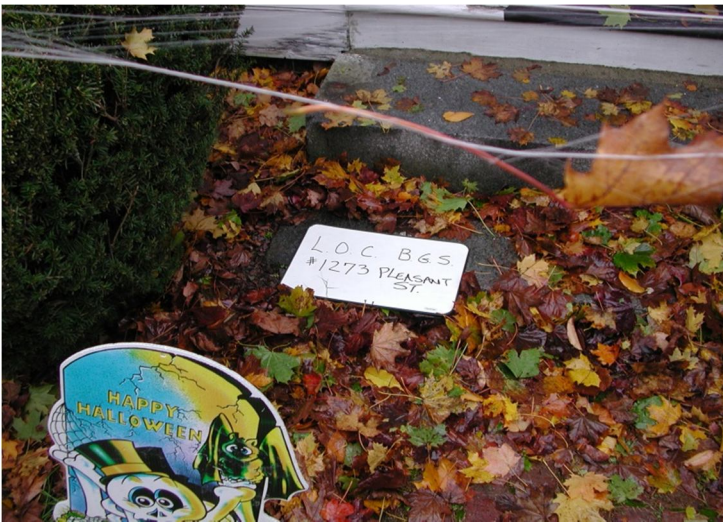
BM LOCBGS 1273 ~ Left Outer Corner Bottom Granite Step @ HSE. #1273 Pleasant St.
